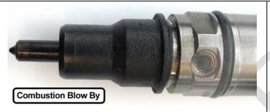
An injector nut that's black with carbon from the chamber gasket to the bottom o-ring, indicates that the sealing surface of the injector sleeve needs to be cleaned. We recommend using solvent and a stiff brush (e.g., Rotunda / Owatonna Tool part number 303-D112) to loosen and remove carbon materials, paying particular attention to the chamber gasket and injector o-ring sealing areas, then use shop towels to clean and dry the sleeve.
