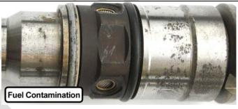
Discoloration, or other visible signs of fuel contamination, in the area between the two injector nut o-rings indicates that the injector has been subjected to water, or other contaminants in the fuel. The fuel should be analyzed to determine if contaminants are currently present (the contaminated fuel that left the evidence may already have flowed through the system). If contaminants are present, a complete flushing of the fuel system is required.
